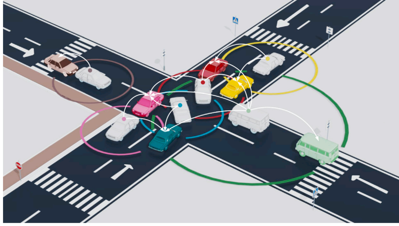
Fig. 3. Dynamic association strategy. Grey-colored car models represent predicted targets, while colored models denote detected targets. Vehicles move in the direction indicated by the gray arrows. The colored rings centered on each prediction represent the association range for the corresponding prediction, where detections covered by the ring are considered potential associations, indicated by white arrows. The color of the dot above each prediction corresponds to the color of its actual associated detection. The proximity between predicted and detected objects reflects the extent of their overlap.
